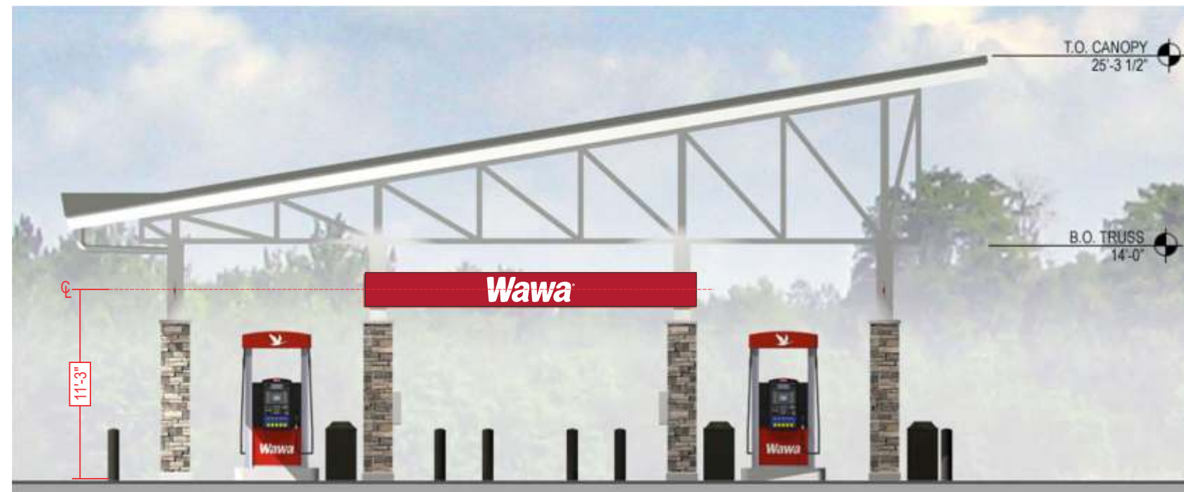
CANOPY END ELEVATION (STACKED PUMPS)
