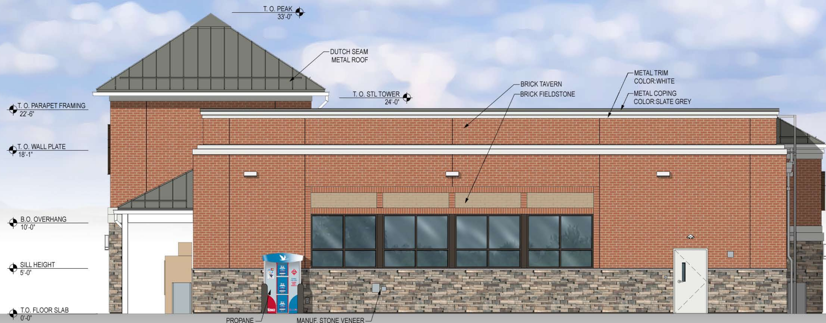
RIGHT (NORTHEAST) ELEVATION (PORT AQUIA DR.)
