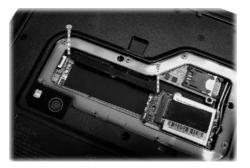
To install the RAM module, match the module's notched part with the socket's projected part and firmly insert the module into the socket at a 20-degree angle (●). Then push down until the retaining clips lock the module into position (●).
