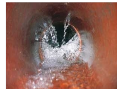
An offset pipe joint showing active Infiltration/Inflow was located during a TV inspection.
