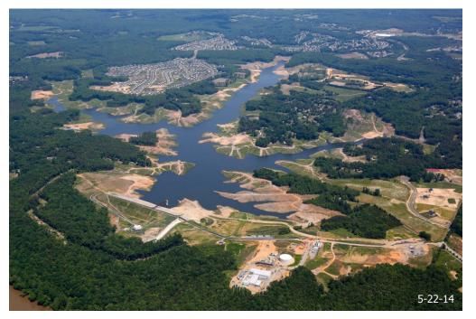
On December 18, 2014. Lake Mooney Reservoir and Water Treatment Facility began operation. Lake Mooney Reservoir is a 40 million gallon per day (mgd) off-stream water storage reservoir with an adjacent water treatment facility. The reservoir was constructed to supply water to the southern end of Stafford County and is the third source of water for the county. Once filled, Lake Mooney will provide a total of 12 million gallons per day.
