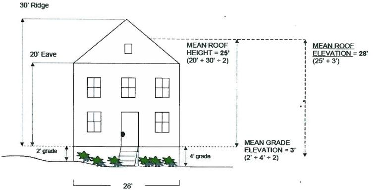
Proposed method for Measuring the height of a Structure
